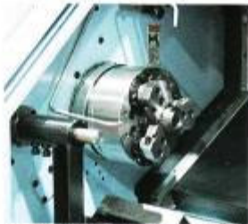
Universal chuck for cast or complex workpieces.
