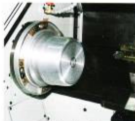
Vacuum chuck for thin workpieces.
