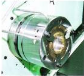
Finger chuck for ring workpiece.
